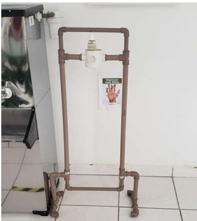
Figure 7: Poços de Caldas Campus hygienic dispenser for gel alcohol produced with PVC pipes.
